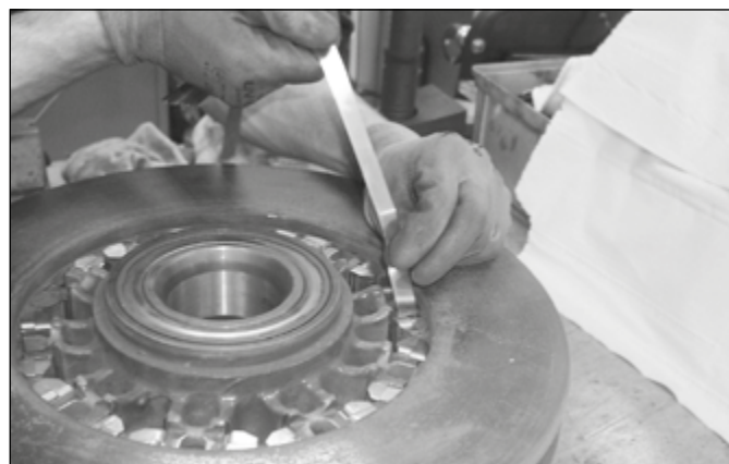
5.4.1.4 - Check radial clearance "S"
