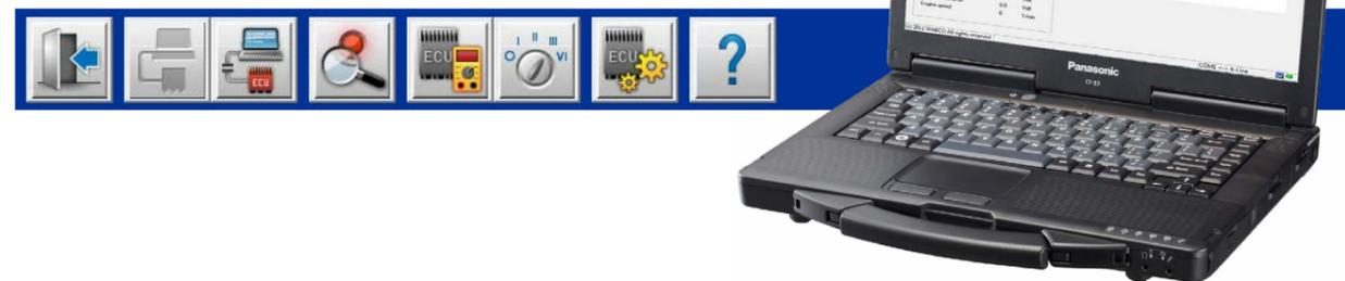
The WABCO diagnostics do not require any special hardware. A standard PC with a free USB port and a Windows XP operating system (or higher) is all you need. We can recommend the WABCO Laptop "Toughbook", a suitable workshop solution which is shock-proof and dirt-resistant. Via the On-Board Diagnostics (OBD) interface in the driver cabin, the PC and the ECU in the truck can be easily connected. WABCO offers matching cables for Daimler vehicles.
