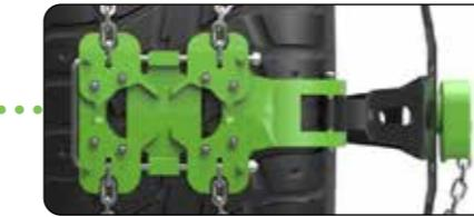
With a link height of only 10 mm, the Tractiva Sport is the lightest and most compact chain in the Tractiva range.
