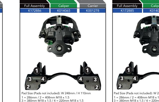
All dimensions are measured from hole centre to hole centre
