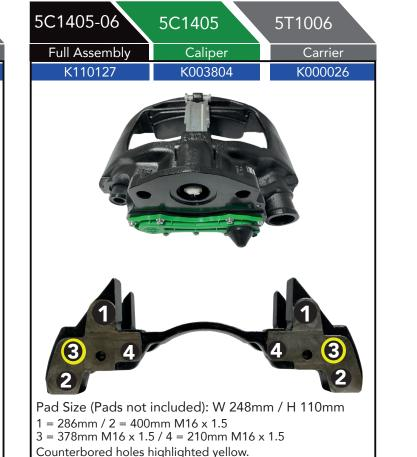
All dimensions are measured from hole centre to hole centre
